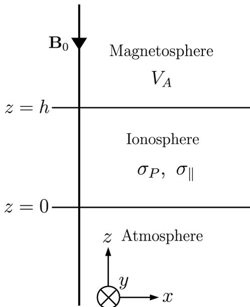
**Figure 1.** Schematic of the model. An ideal magnetosphere characterised by an Alfvén speed  $V_A$  is situated above a distributed ionosphere ( $0 < z < h$ ). The system is driven by an incident Alfvén wave with fields  $E_{xi}(x)\hat{\mathbf{x}}$  and  $b_{yi}(x)\hat{\mathbf{y}}$ . The solution is invariant in the  $y$  direction.
