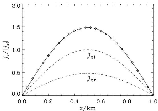
**Figure 6.** The variation field-aligned current at the magnetosphere-ionosphere interface with  $x$  for  $\lambda = 2$  km. The solid line is  $j_z^-$  and the symbols  $j_z^+$ . (Other parameters are the same as in Figure 2.)
