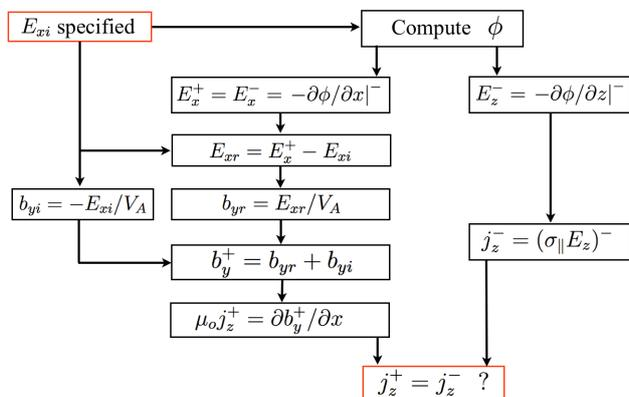
**Figure 5.** Flow chart outlining the current consistency check. Given the incident wave ( $E_{xi}$ ) there are two routes to calculate  $j_z$  at the interface: one through the magnetosphere ( $j_z^+$ ) and the other through the ionosphere ( $j_z^-$ ). For an accurate self-consistent solution these will be the same to within the accuracy of the solution.
