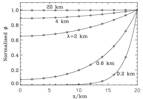
**Figure 3.** The variation of  $\phi$  with altitude across the ionosphere (normalised by the value at  $z = h^-$ ). Results are shown for horizontal wavelengths of 0.2, 0.6, 2, 4, and 20 Km. The solid lines are numerical results and the symbols represent the analytical solution (25) which varies as  $\cosh(\sqrt{\sigma_P/\sigma_{\parallel}} 2\pi h/\lambda)$ . (Parameters are the same as Figure 2.)
