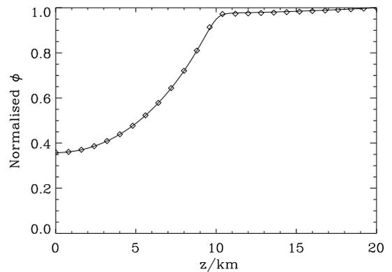
**Figure 4.** A similar format plot to Figure 3, except that  $\sigma_{\parallel}$  jumps from a value of 0.02 mho/m ( $0 < z < 10$  km) to 2 mho/m ( $10 < z < 20$  km). The horizontal wavelength is 2 km. Other parameters are the same used in Figure 2.
