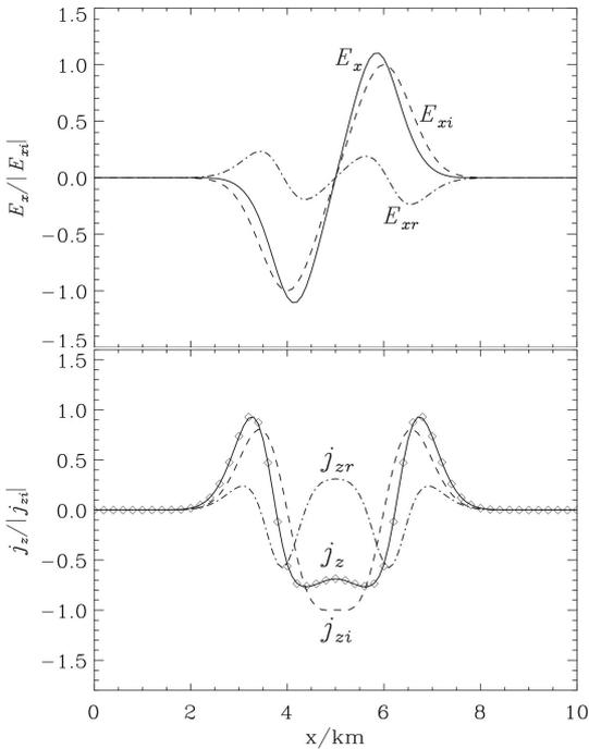
**Figure 9.** A similar format to Figure 7. The incident Alfvén wave and parameters used to generate the results in Figures 7 and 9 are the same except Figure 9 used the  $\sigma_P$  distribution displayed in Figure 8, whilst Figure 7 used a uniform  $\sigma_P$  of  $5 \times 10^{-4}$  mho/m. Note how the reflected fields over the downward current region ( $4 < x < 6$  km) differ between Figures 7 and 9, and hence the total  $E_x$  and  $j_z$  are also modified there.
