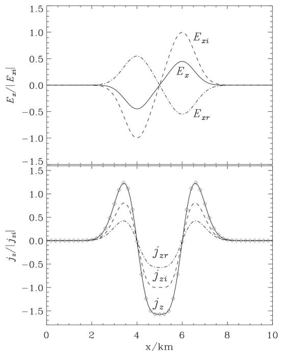
**Figure 7.** The variation of  $E_x$  and  $j_z$  at the magnetosphere-ionosphere interface ( $z = h$ ) with  $x$ . The total  $j_z$  consists of a strong downward current that closes in two adjacent smaller upward currents. Both  $j_z^+$  (symbols) and  $j_z^-$  (solid line) are shown. Parameters are the same as in Figure 2.
