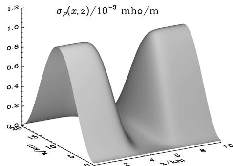
**Figure 8.** A surface plot of nonuniform  $\sigma_P(x, z)$  with conductivity depleted below the downward current. In the undepleted regions the height-integrated Pedersen conductivity is similar to that employed in constructing the results shown in Figure 7.
